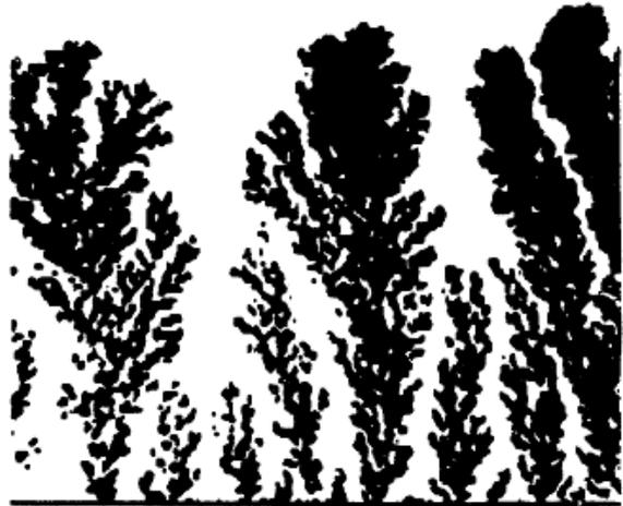
**Figure 6:** Digitized growth pattern of copper deposited at an electrode potential of -5V from solution of  $\text{CuSO}_4$  with concentration 0.05 after the elapsed time of 10 min. [13].
