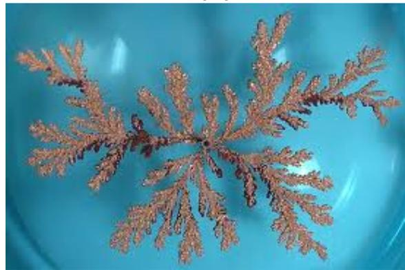
**Figure 7:** A typical DLA cluster grown from a copper sulfate solution in an electrodeposition cell [1].
