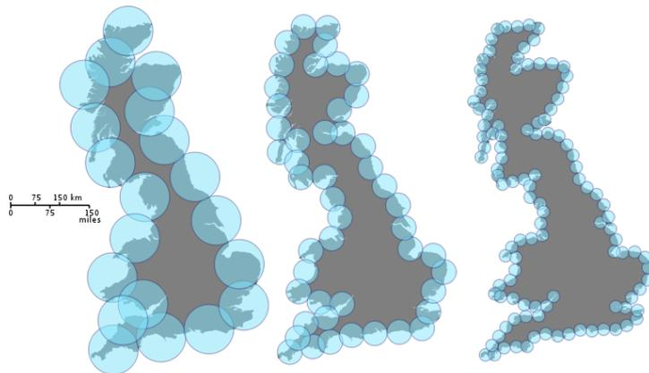
**Figure 3:** Measuring the length of the shore of England. Decrease of the sizes of the measuring devices (spheres) leads to the infinitely large length but infinitely small area [1].
