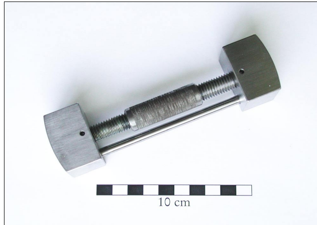
Figure D.2: Picture of steel substrate used as counterpart for the probe, when measuring the thickness of the beam pipe windows. The nut is used to adjust the distance between the two steel blocks, until they fit closely to the inner wall of the beam pipe.
